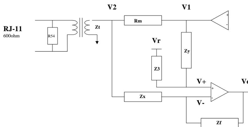
Figure 1: General representation of Telco interface network.
