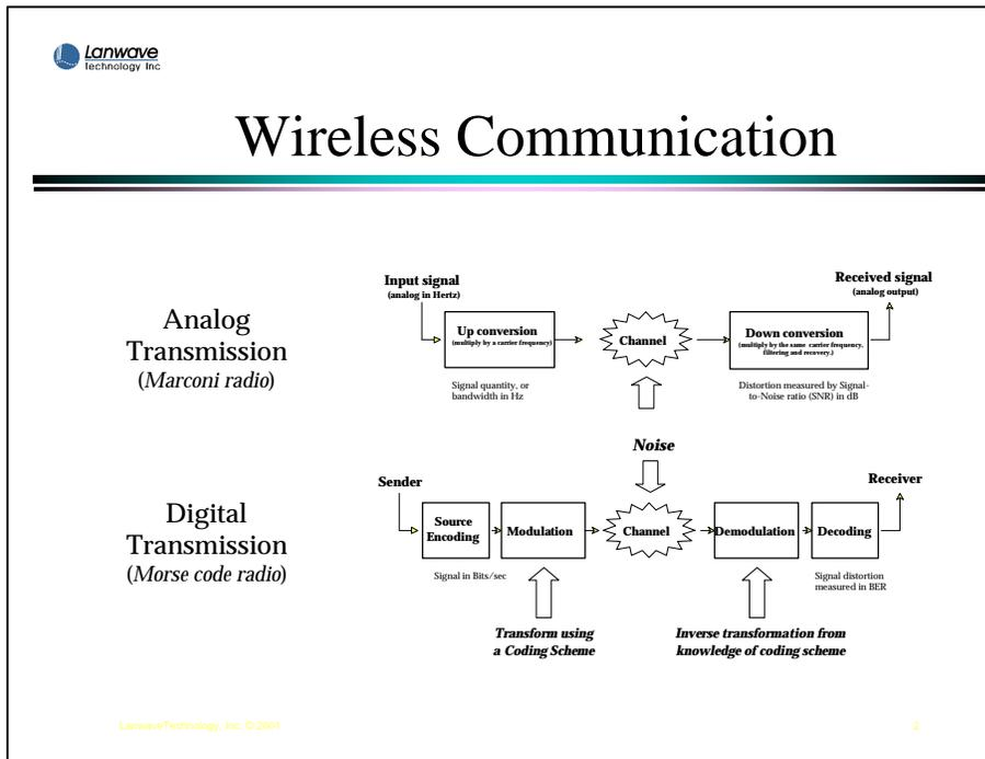
The primary difference between analog and digital transmission is in the addition of a coding engine known as the **wireless DSP base band chip**. In the cordless phone and similar voice devices, a second **voice DSP chip** for source digitization and information compression is used. Lanwave provides both chips and their collateral software to our customers.
